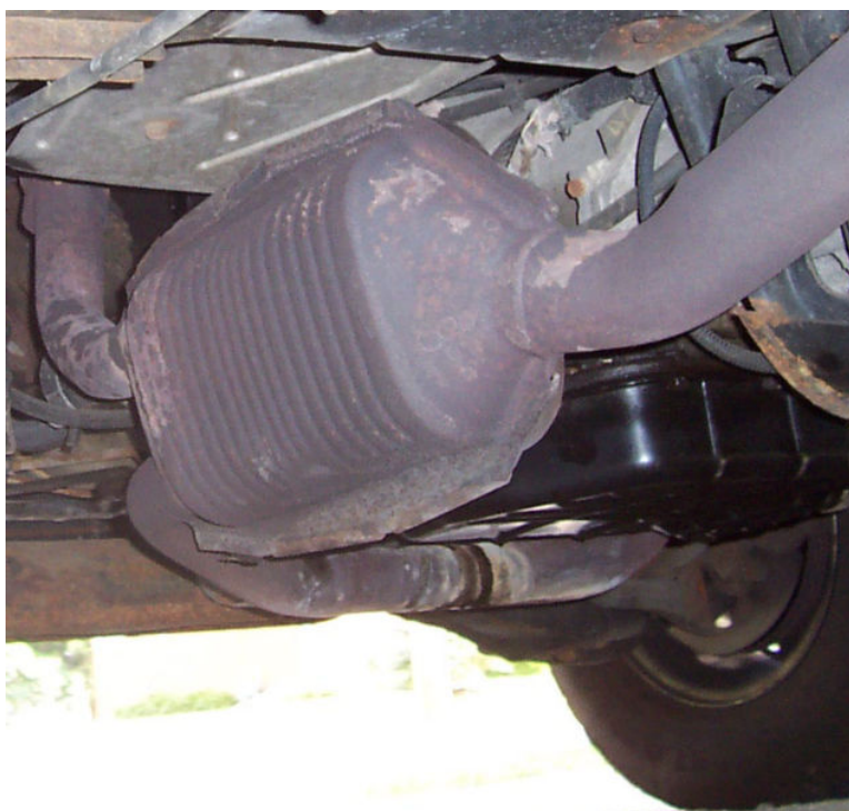
Figure 22.12: A large catalytic converter on an SUV. (11)
