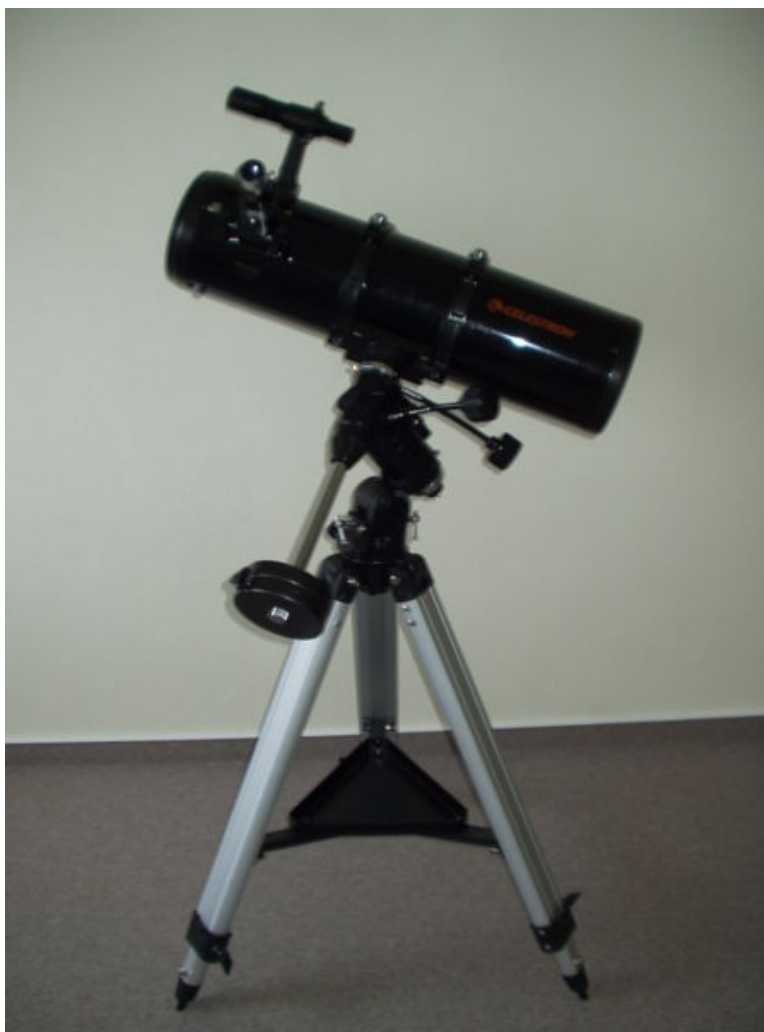
Figure 23.6: Reflecting telescopes used by amateur astronomers today are similar to the one designed by Isaac Newton in the 17 th century. (13)
