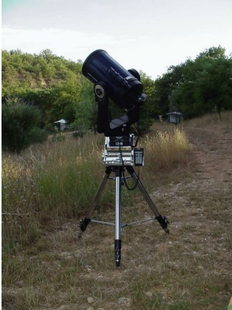
Figure 23.8: Many amateur astronomers today use catadioptric telescopes. These telescopes have large mirrors to collect a lot of light, but short tubes for portability. (34)
