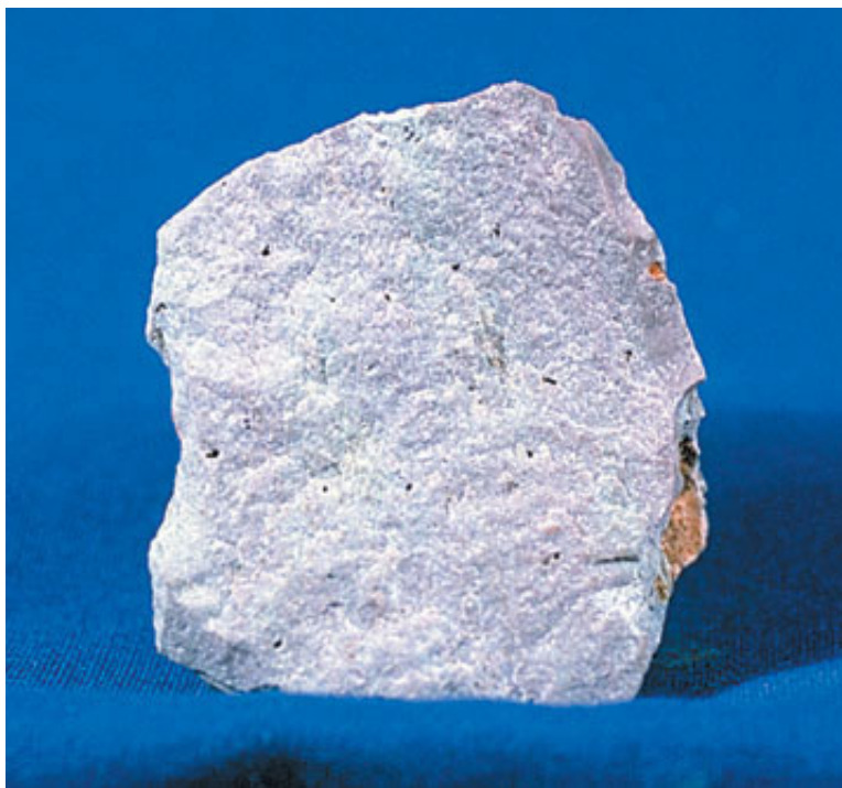
Figure 3.21: Rhyolite rocks contain minerals that are similar to granite, but the crystal size is much smaller. (18)
