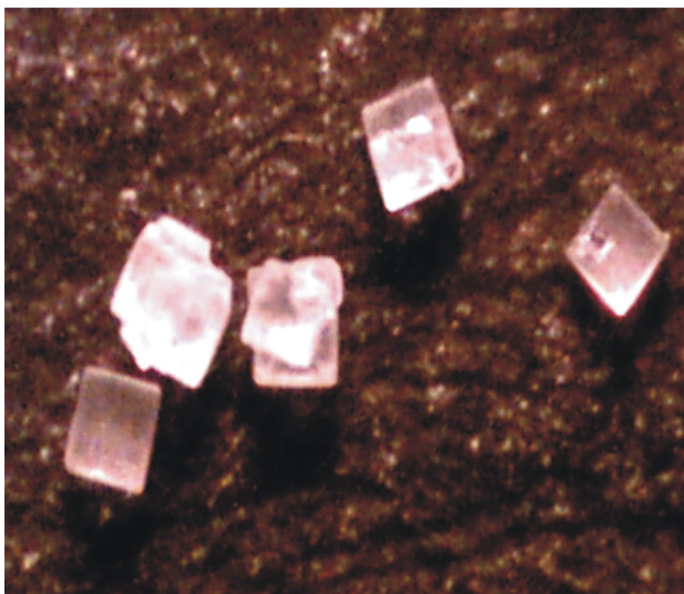
Figure 3.4: When you look at grains of table salt under a microscope, you can see that the crystals are made of square shapes. (32)
