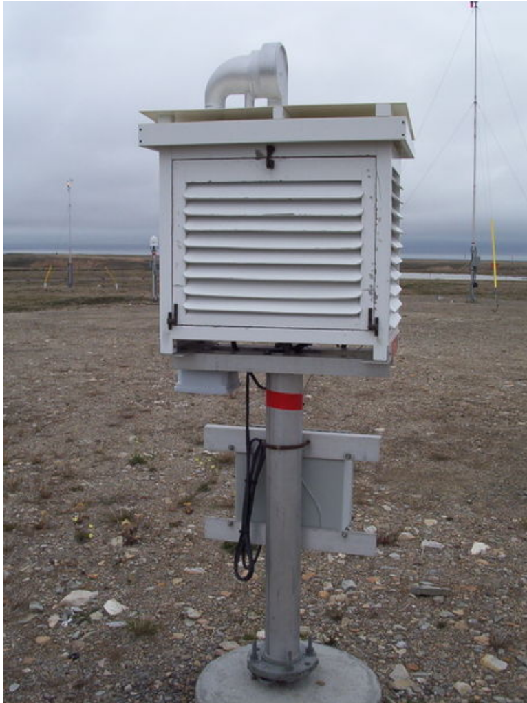
Figure 16.39: A land-based weather station. Since some of the instruments must be protected from precipitation and direct heat, they are held behind a screen. (38)
