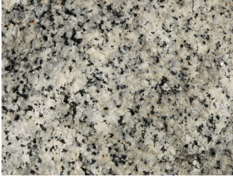
Figure 4.12: A close-up of a granite sample. Notice the black and white portions. Each color represents a different mineral in the rock. You can easily see the mineral crystals that make up this intrusive igneous rock. (22)
